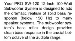
The subwoofer system's effect is most dramatic when it is combined with mini-speakers. The mini-speakers reproduce the high, mid-range, and upper bass frequencies, while the subwoofer reproduces the low bass frequencies. This results in heightened presence and clarity for the entire audio range.
